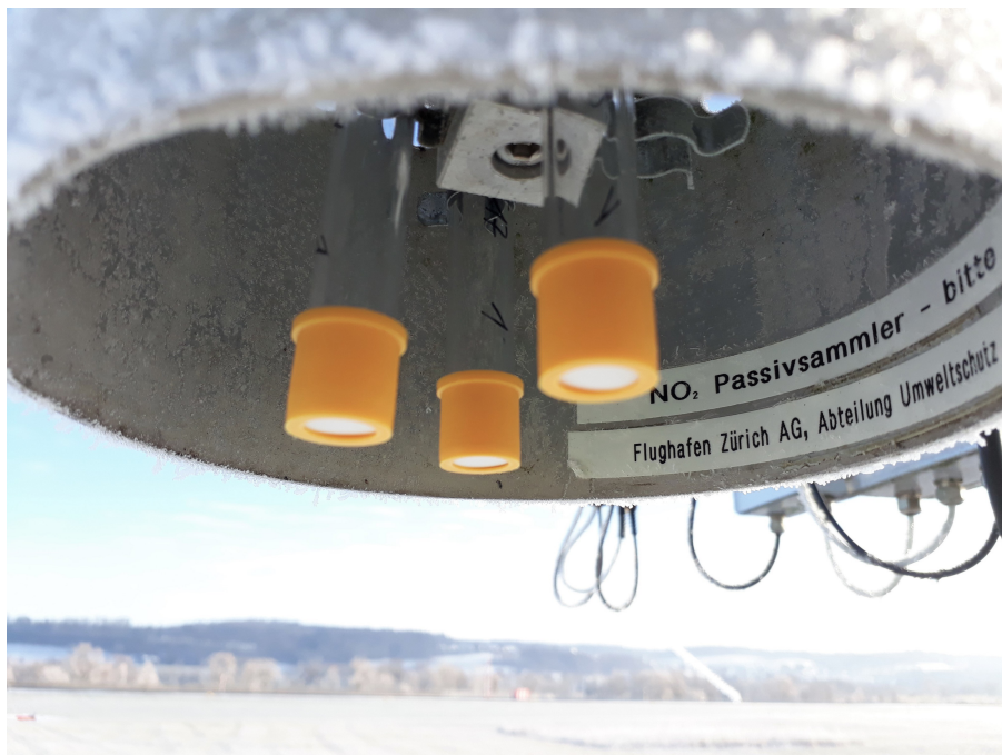
Passive collectors are used to measure the concentration of nitrogen dioxide.
